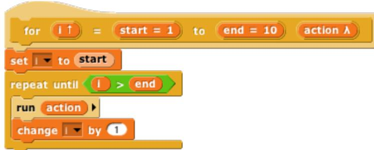
This is simplified because it assumes, without checking, that the ending value is greater than the starting value; if not, the block should (depending on the designer’s purposes) either not run at all, or change the variable by  $-1$  instead of by  $1$ . (The **for** block in **Snap!**’s tool library works for ascending or descending values; you can read its script by right-clicking or control-clicking on it and selecting the Edit option.)
